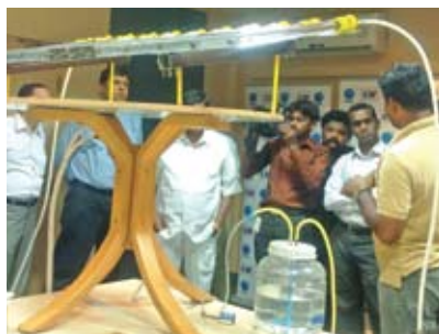
Solar Water Purifier with integrated supply and storage system for rural areas
